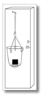
One by one, place each known mass into the cup and make a pencil mark on the board next to the rim. Write the mass value next to the mark.
