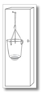
We will calibrate the device by putting objects of different, known masses into the cup. As we put each mass into the cup, the mass will be pulled down by gravity, taking the cup with it.
