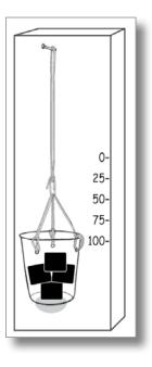
The principle here is that the greater an object's mass, the greater the effect gravity has on it. Each object is pulled down the board a distance that is directly related to the amount of its mass.
